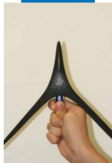
Empirical test of Plastimul 2K Reactive's high flexibility and resistance to punch loads
