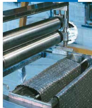
Impregnating MapeWrap C with a machine
