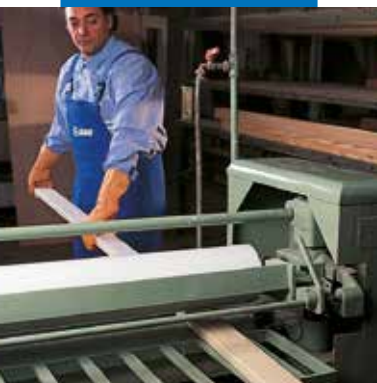
Applying Adesivil D3 with a roller to bond wood sections
